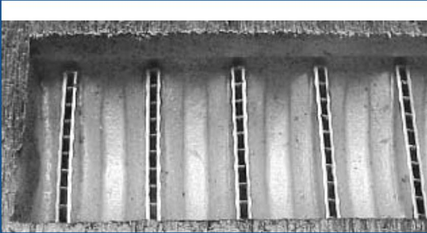
*Cutaway View of Parallel Flow Condenser Tubes*
