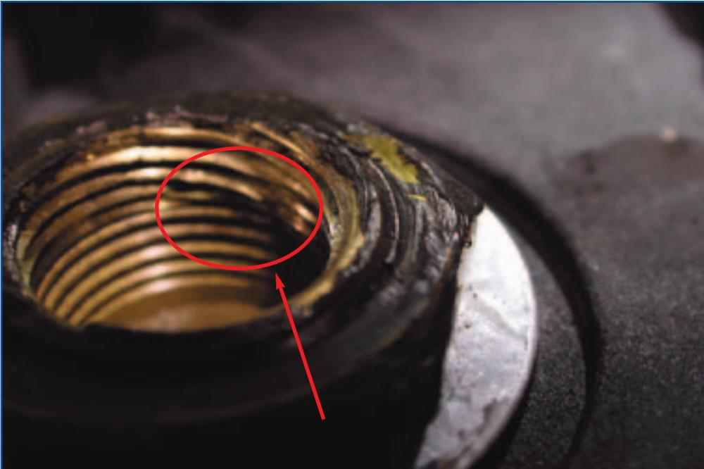
***Stripped oil cooler threads***
